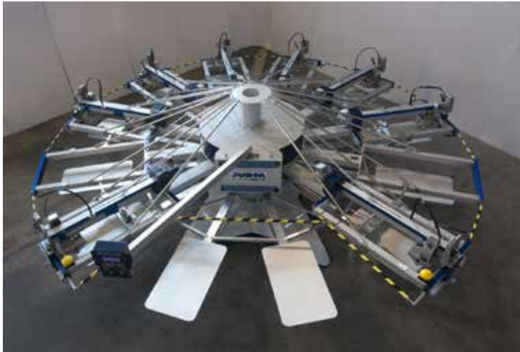
MHM's Synchroprint X-Type Automatic Screenprinting Press has a revolutionary AC indexing system and a high power AC electric printhead drive that translates into very fast printing speeds. The X-Type also features individual off contact front and rear adjustments, which are critical when printing high density or other specialty inks, separate squeegee and flood blade air pressure regulators which provide greater squeegee pressure control, and a time-saving preregistration screen system featuring the MHM pinlock.
